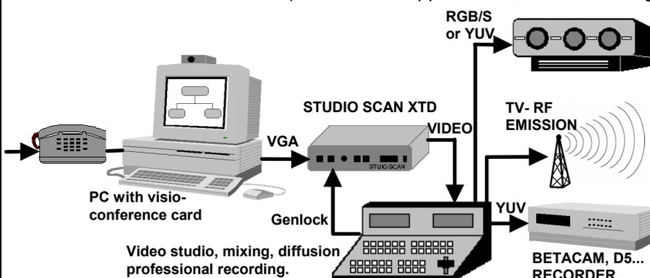
The ANALOG WAY scan converter **STUDIO SCAN XTD**, is dedicated to the professional broadcast applications. It allows to diffuse Visio Conference images in video "live" studios with a YUV, RGB/S, S.VIDEO, PAL or NTSC standard and with the possibility for the converter to be locked into the video studio (Genlock).
