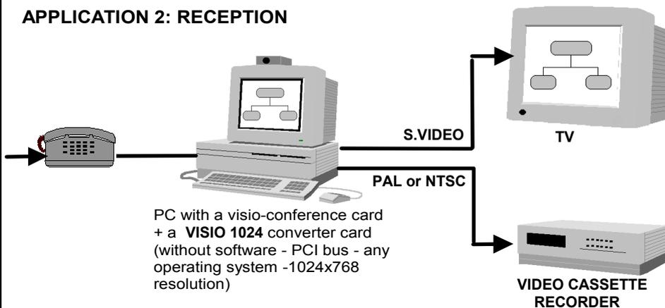
The **VISIO 1024** scan converter card allows to display on a TV screen or to record on a video tape a Visio-conference communication.
