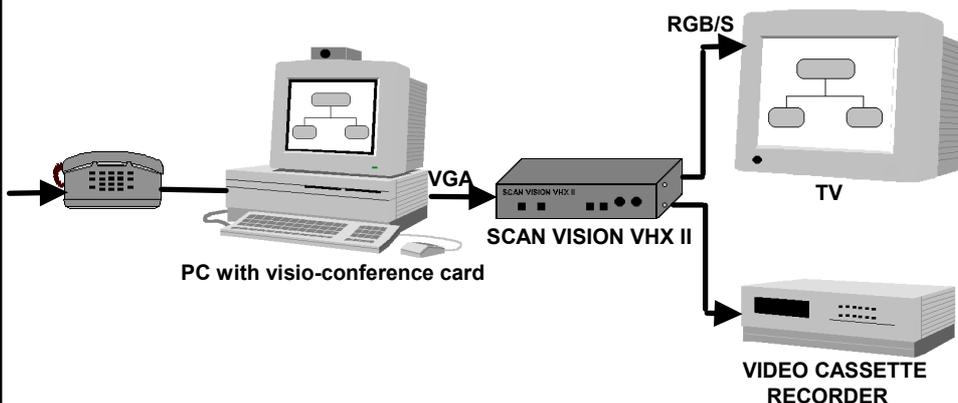
The ANALOG WAY scan converter **SCAN VISION VHX II**, allows to convert all computer signals from PC or MAC to TVs (with a RGB/S connection for a maximum quality) and to record a visio-conference communication on a videotape (VHS, S-VHS, Hi-8).
